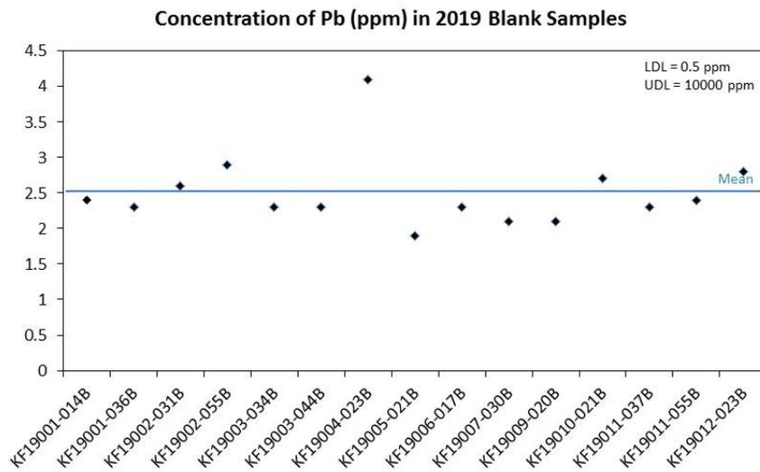
**Figure 11-4k: Blank material analyzed by ALS in the 2019 Knife Lake DDH core shipments - Pb**
