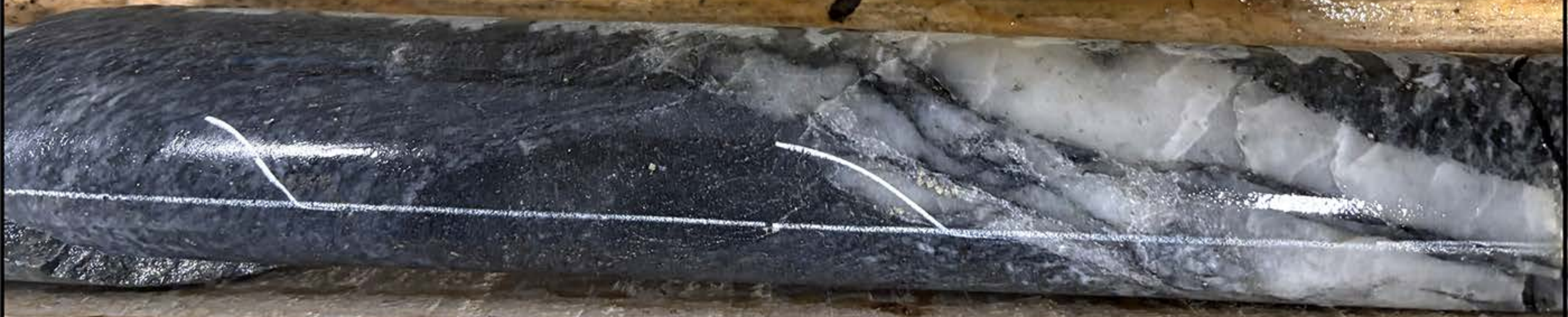
CL26032 361.4m sheared qtz-carb vein (38.1 g/t Au)
